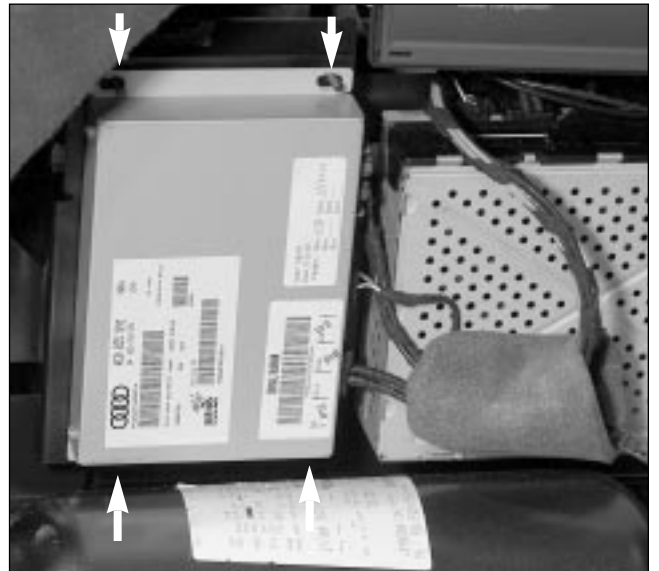
Step#8 Attach Satellite Radio Receiver unit to bracket using 4 self locking nuts. Torque to 3 Nm. Ensure that all wires are routed properly to prevent damage to wiring and the fiber optic cable.
